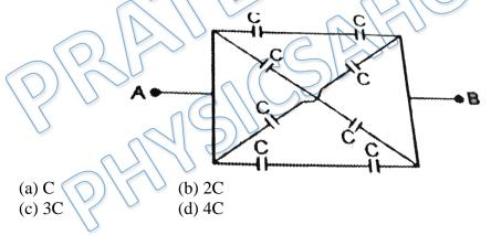
Q 12. Calculate the equivalent capacitance between the points A and B of the circuit given below.
